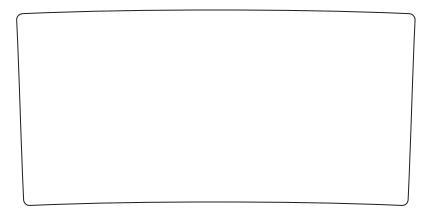
Artwork Design: Use rectangle shape 2.0" x 4.0", 1/16" Corner Radius Curvature will be applied by SpectraGraphics
