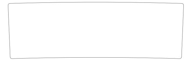
Artwork Design: Use rectangle shape 1.875" x 5.875", 1/16" Corner Radius Curvature will be applied by SpectraGraphics
